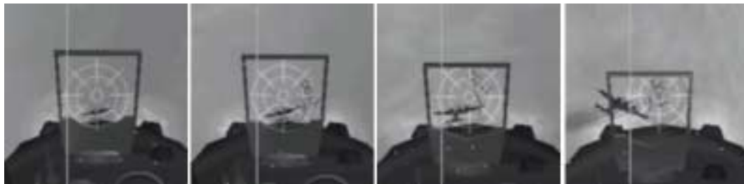
Fig 18. In the sequence above, a 110 is vainly trying to outzoom a Curtiss Hawk who cuts across his circle and fires a long burst from range 400 (first frame) down to range 200 (last frame). The amount of deflection and the effects are clearly visible.
